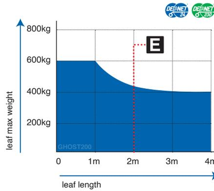
If the leaf length is bigger than 2m or if you use reversible models you must install the electric-lock to block the gate in closed position. The height and the leaf structure, as well as the presence of strong wind, can cause the reduction of the value of the data contained in table or make it necessary to use an electric lock also for leaves shorter than 2m.
