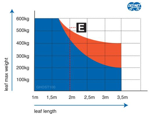
If the leaf length is bigger than 2m or if you use reversible models you must install the electric-lock to block the gate in closed position. The height and the leaf structure, as well as the presence of strong wind, can cause the reduction of the value of the data contained in table or make it necessary to use an electric lock also for leaves shorter than 2m.
