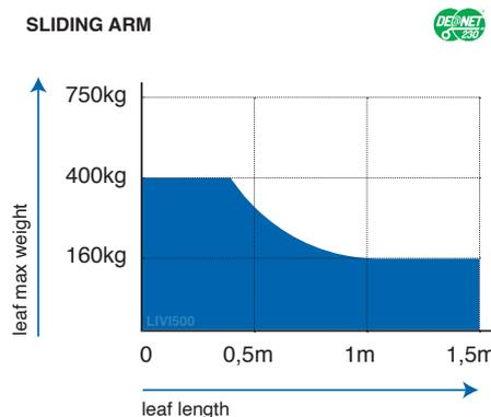
The electric-lock must be fitted to block the gate in closed position. The height and the leaf structure, as well as the presence of strong wind, may cause the reduction of the value of the data contained in table.
