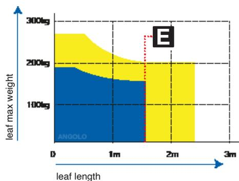
If the leaf length is bigger than 1,5 metres or if you use reversible models you must install the electric-lock to block the gate in closed position. The height and the leaf structure, as well as the presence of strong wind, can cause the reduction of the value of the data contained in table.
