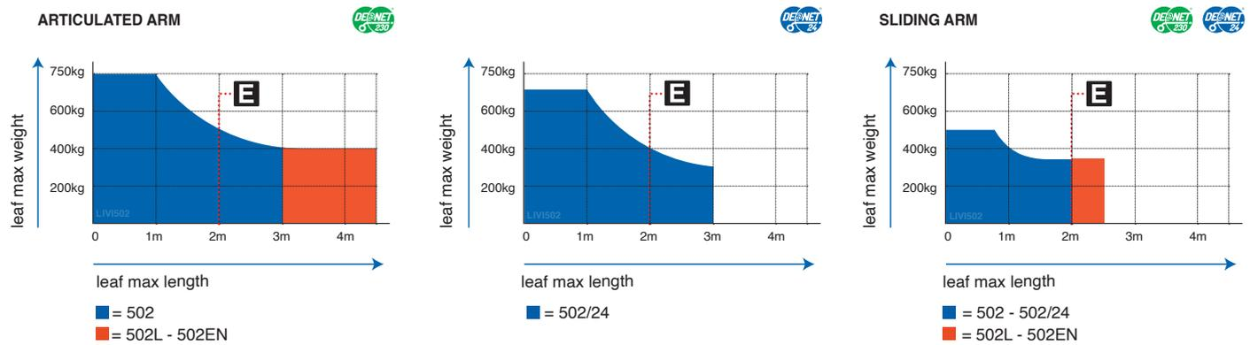
If the leaf length is bigger than 2m or if you use reversible models you must install the electric-lock to block the gate in closed position. The height and the leaf structure, as well as the presence of strong wind, can cause the reduction of the value of the data contained in table or make it necessary to use an electric lock also for leaves shorter than 2m.
